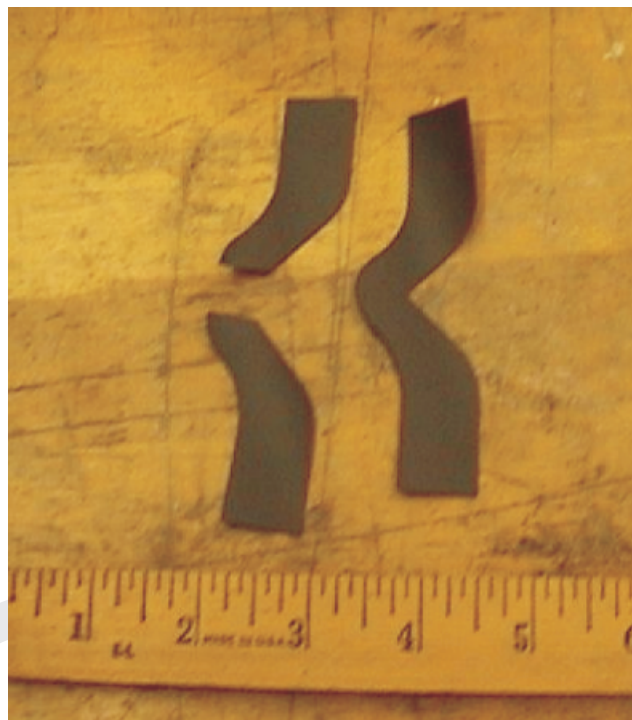
Figure 11. Tear specimens after and before testing
