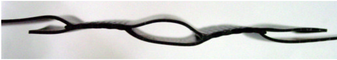
FIG. 2. Exaggerated view of an inflated dual track PVC geomembrane thermal weld produced with a Leister Twinny hot air welder.
